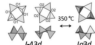
$\text{RbBSi}_2\text{O}_6$  25 °C  $I\bar{4}3d$   $a = 12.785364(70)$  Å
